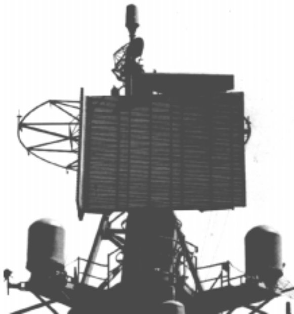
Figure A82 AN/SPS-48 frequency-scanning 3D radar antenna.
