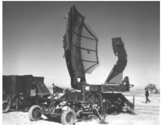
Figure A76 AN/TPS-43 stacked-beam reflector antenna.
