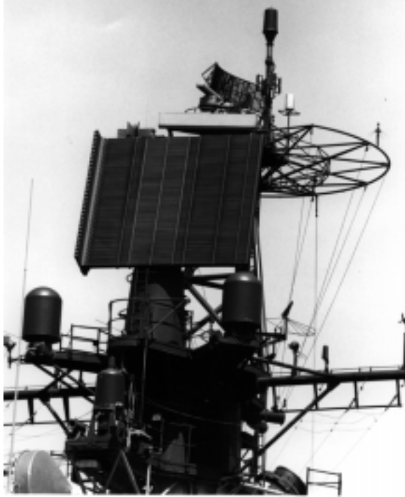
Figure R66 AN/SPS-48 multiple-beam scanning 3D radar (ITT Gilfillan photograph).
