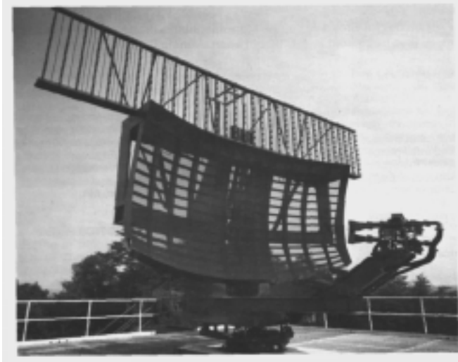
Figure R8 ASR-9 radar antenna (from Skolnik, 1990, Fig. 6.14, p. 6.19).
