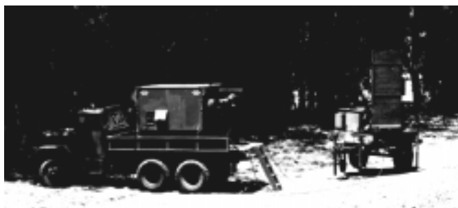
Figure R12 AN/TPQ-36 mortar location radar (Hughes Aircraft Co. photo).
