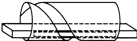
Figure S7 Helical-slot scanner (from Johnson, 1984, Fig. 18.29, p. 18.25, reprinted by permission of McGraw-Hill).
