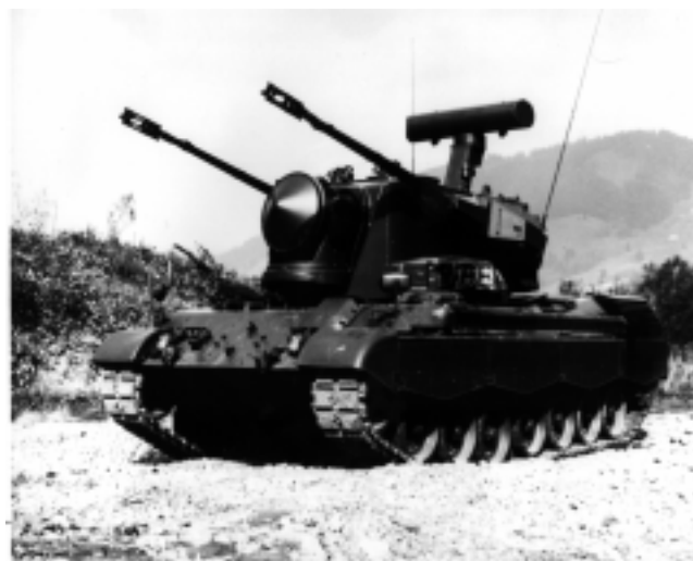
Figure R29 Flakpanzer anti-aircraft tank system. The K a -band fire control tracker shares the forward antenna with a longer range X-band tracker, whose transmitter also serves the target acquisition radar at the rear of the turret.
