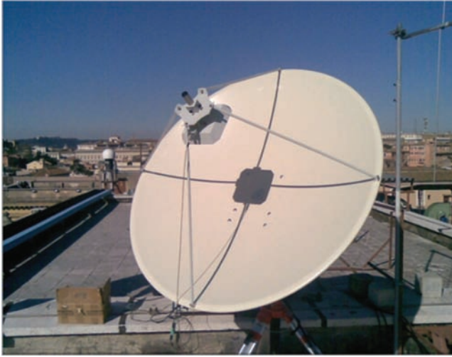
Figure 15.13 Parabolic antenna exploited at the reference channel for the experimental DVB-SH based PR Rx
