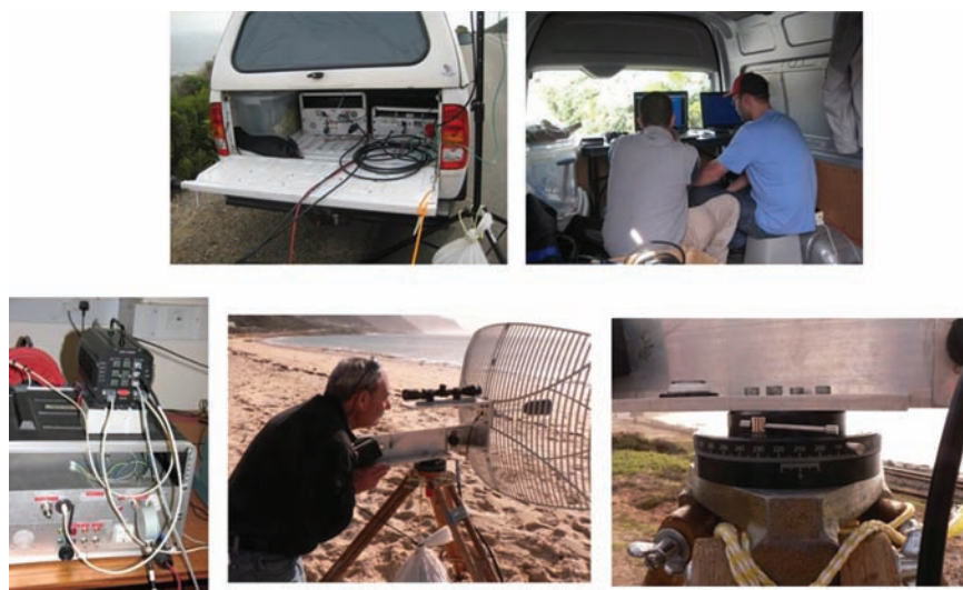
Figure 12.20 Pictures of the NetRAD multistatic radar system in use in trials. Clockwise from top left: transmit equipment in van; operator position; vernier scale for antenna alignment; telescope for antenna alignment; GPSDO
